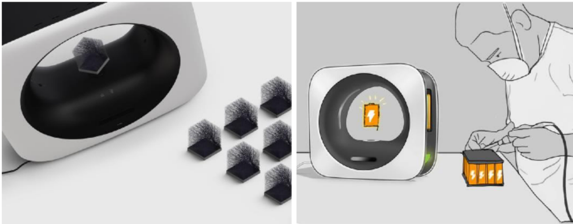
Figure 6 (a) biomA 3D prints organic batteries from algae and chitosan biopolymer. (b) Designed for local production and consumption with prosumers. Credit: Jomy Joseph
