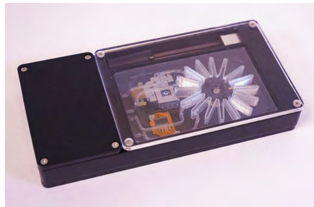
Figure 10 a) A Biomineralising rig. b) Biomining cartridges that harvest rare-earth for community biomining. Images by Vahidi et al., (2118)
